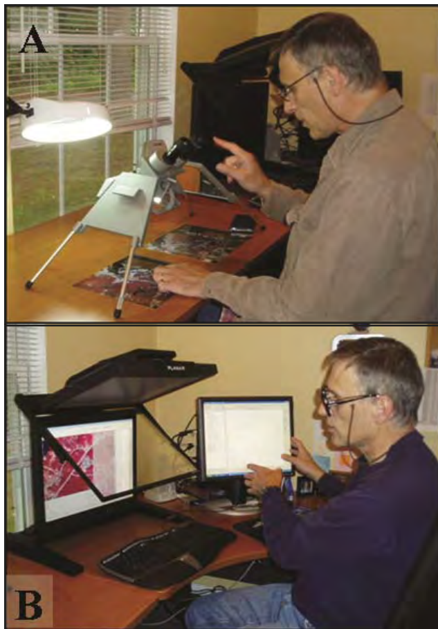
Figure 13: Photo interpretation. A) Using paired 9 x 9 inch stereo contact prints viewed under a mirror stereoscope. B) Using digitized aerial photographs viewed on-screen in 3-D.
